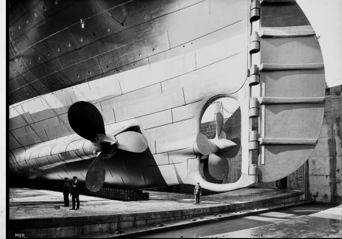
Above: Workmen are dwarfed by the port and centre propellers of Olympic in the graving dock at Belfast in April 1911.
