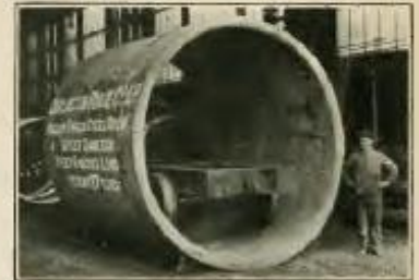
HOLLOW FORGED STEEL DRUM. 10 feet diam. 9 feet 6 inches long. Weight, 27 tons.
